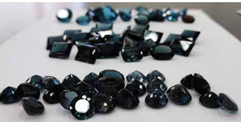
Photos of semi-precious topazes: - natural colour (top); - coloured by irradiation in a reactor (bottom)
